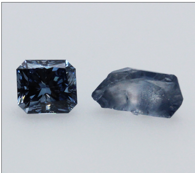
Fig. 7a: Two synthetic fancy blue diamonds, produced by HPHT (NDT). The left is a faceted synthetic of 0.56ct (VS2 clarity) and on the right a crystal of 0.67ct. Both are type IIb synthetic diamonds (both stones part of GRS reference collection). Photo by Matthias Alessandri.
