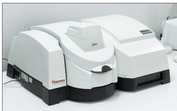
Fig. 1 Modern UV-Vis-NIR unit. Note the wide standardized compartment designed to accommodate the most diverse sampling setup required in various fields of application.
